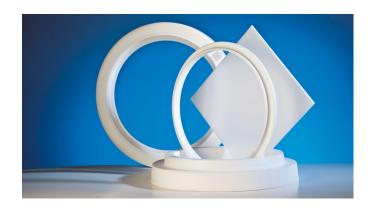
OM® 100 features the typical viscosity and thermal properties of high purity quartz glass. Due to its high density OM® 100 can be easily welded to clear fused quartz with excellent welding seam quality. The mechanical strength is almost equivalent to clear fused quartz and superior to most competing materials.
